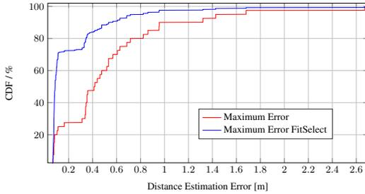
**Fig. 3:** Cumulative distribution function (CDF) of maximum distance error in  $\mathbf{A}_p$  and selected subset of  $\mathbf{A}_p$  by FitSelect function.
