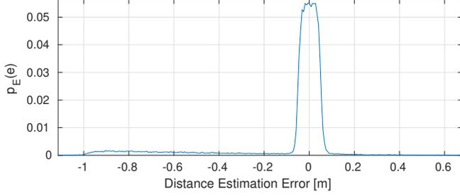
**Fig. 2:** Histogram of distance estimation errors from 80.000 observations.
