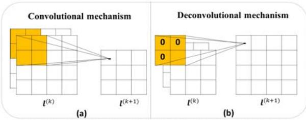
Fig. 3 (a) Convolutional and (b) deconvolutional operations.
