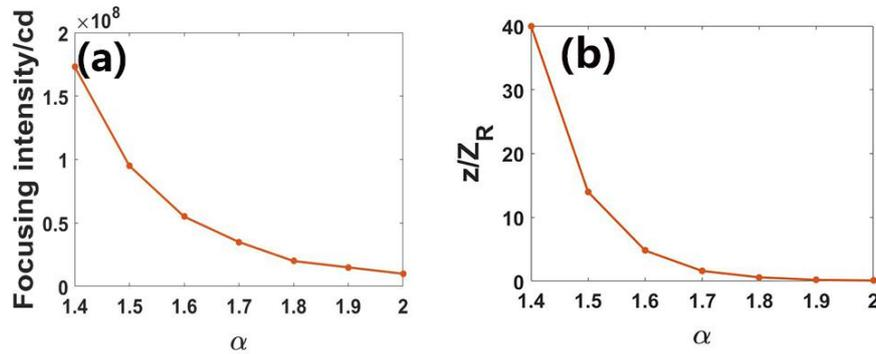
Fig. 6. (color online) (a) and (b) are the focal intensity and the focal length under different Lévy indexes, respectively. Other parameters are the same as those in Fig. 5.
