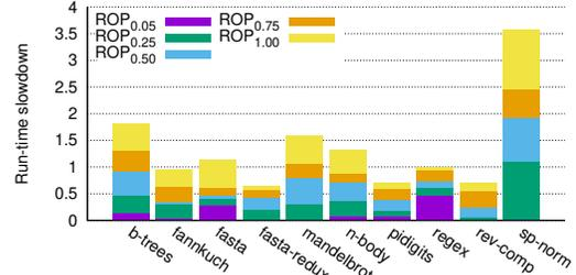
Fig. 5: Run-time overhead for `clbg` benchmarks of different ROP $_k$  settings with 2VM-IMP<sub>last</sub> used as baseline.
