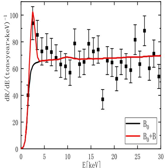
FIG. 1. Fit to the observed data [1] about the number of events  $dR/dE$  ( $\text{ton year keV}^{-1}$ ) as function of the reconstructed electron recoil energy with five different sets of benchmark values C1 to C5 in Table.I, where  $B_0$  and  $B$  represents the background and the daughter DM contribution, respectively.
