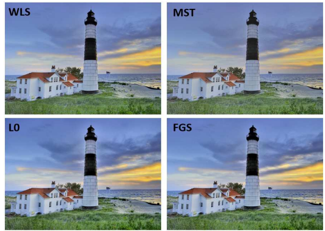
Fig. 8: Detail enhancement using equivalently smoothed images (50% gradient reduction). L0 and FGS exhibit some darkening in the grass texture, and have stronger halos.
