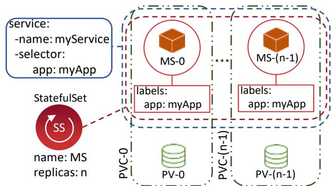
Fig. 1. Deploying stateful applications with StatefulSet controllers.
