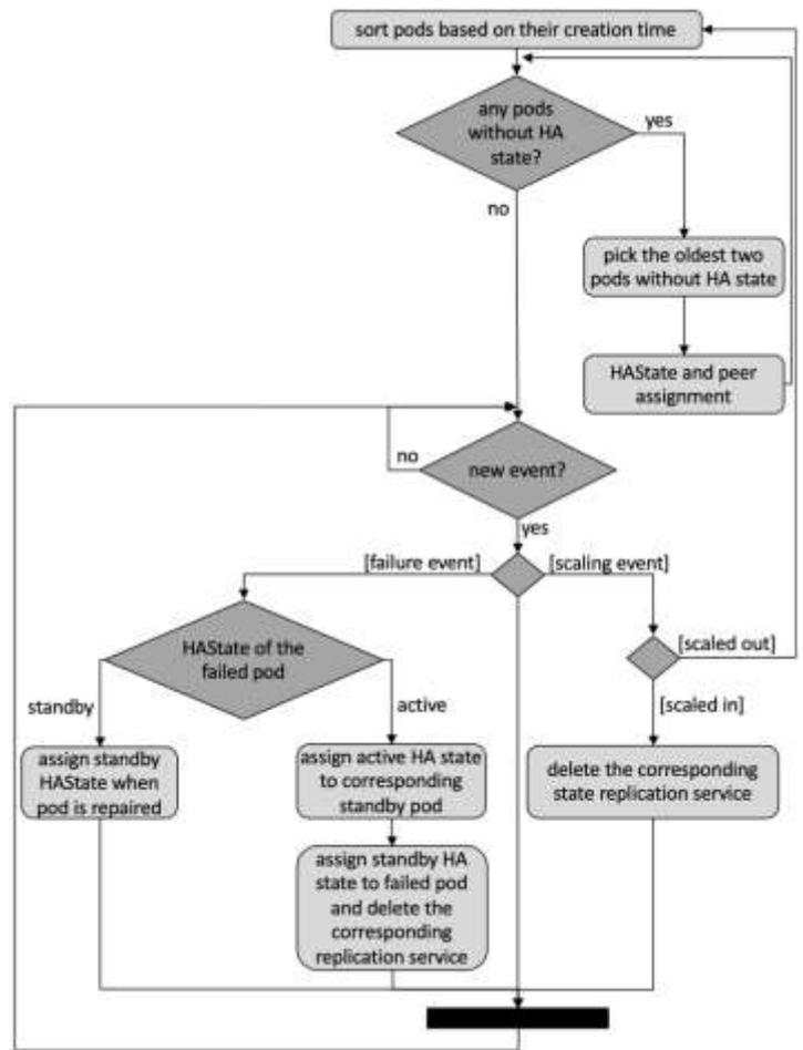
Fig. 3. Activity diagram of the HA State Controller.
