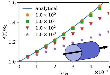
Figure 3: Pipe erosion with a constant pressure drop as a function of the dimensionless time. The different colors and markers correspond to different erosion rates. The erosion threshold is zero and the initial radius of the tube is  $R_0 = 32$ , schematized in the inset. The analytical result, Eq. (22), is plotted with a blue line.
