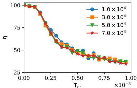
Figure 7: Removal efficiency for the porous medium composed of circular obstacles with a constant flow rate  $Q = 2.56$ . Different colors and markers correspond to different timescales of swelling.
