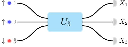
Figure 3: An  $N = 3$  LQN with a tritter. Two bosons with  $\uparrow$  are injected to input modes 1 and 2, and a boson with  $\downarrow$  is injected to 3. The total transformation matrix  $U_3$  is unitary as Eq. (16), and we postselect no-bunching states (one particle per output detector  $X_j$ ,  $j = 1, 2, 3$ ).
