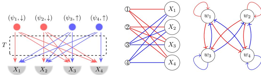
(a) An  $N = 4$  LQN. Each particle, initially at  $\psi_i$  (spatial wavefunction,  $i = 1, 2, 3, 4$ ), evolves by the linear transformation operator  $T$  and arrives at the detectors  $X_i$  ( $i = 1, 2, 3, 4$ ). The blue (red) color denotes the internal state  $\uparrow$  ( $\downarrow$ ).
