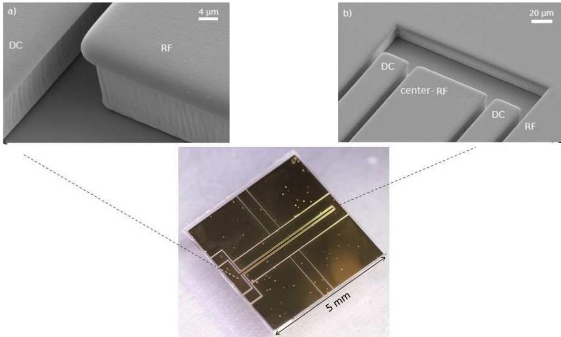
**Figure 4.** A 5 x 5 mm<sup>2</sup> trap chip made of gold structures with high aspect ratio (5:1) electroplated on sapphire. a) SEM micrograph of a control DC electrode and an RF electrode separated by an effective gap of 4 μm. b) SEM micrograph of an outermost part of the chip showing part of the RF and DC trap electrodes.
