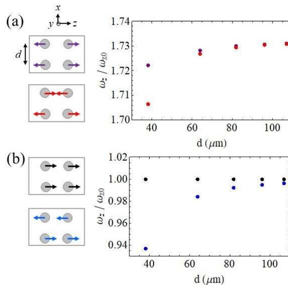
**Figure 3.** Ion motion and corresponding eigenfrequencies of (a) stretch modes and (b) COM modes in the  $z$  direction of  $2 \times 2$   $^{40}\text{Ca}^+$  ion crystals. The distance between two ion strings is indicated by  $d$ . A confinement with  $\omega_{z0}/2\pi$  of 0.19 MHz is assumed for the calculation. The eigenfrequencies  $\omega_z$  are normalized by  $\omega_{z0}$ .
