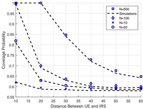
Fig. 3: Coverage probability as a function of the IRS elements  $N$  when  $m = 0.5$ ,  $\alpha = 4$ ,  $\theta = 5$ dB,  $r = 500$  m,  $p = 2.5$  W (The blue data points are obtained from analysis. The dotted black lines are obtained from simulations).
