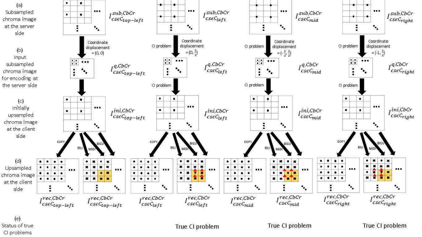
Fig. 5. The proposed flow diagram to analyze the CI problem for all combinations in CSxCU. (a) Subsampled chroma image. (b) Input subsampled chroma image for encoding. (c) Initially upsampled chroma image. (d) Upsampled chroma image. (e) Status of true CI problems.
