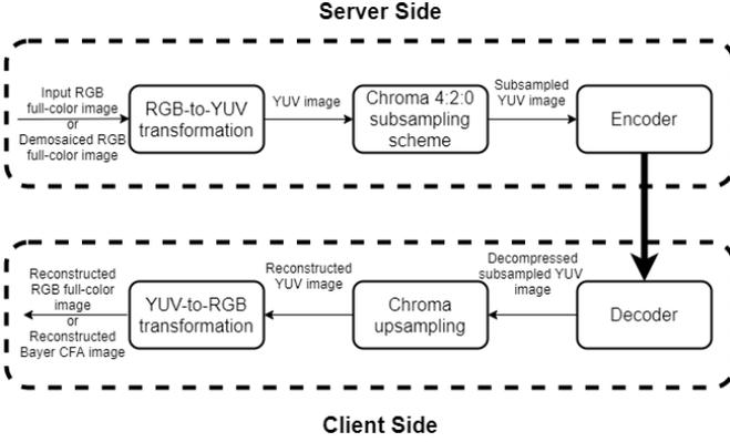
Fig. 1. The current coding system.
