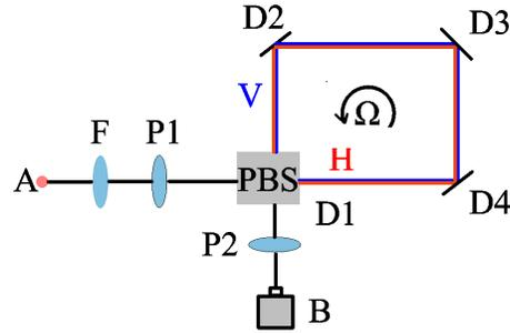
Fig. 2: Schematic of the modified Sagnac's interferometer based on weak measurements. A=light source; B= observer (the spectrometer) ; D1, D2, D3 and D4 are common mirrors; F is the Gaussian Filter; P1 is the polarizer corresponding with preselection, P2 is the polarizer corresponding with postselection.
