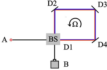
Fig. 1: Schematic of Sagnac's interferometer. A=light source; B= observer; BS = beam splitter ; D1 and D2 are common mirrors; D3 is a special curved mirror
