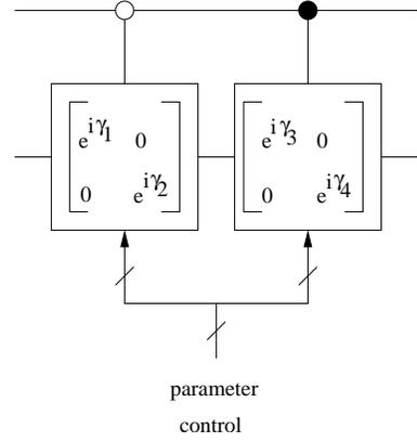
FIG. 5. Implementation of quantum operator defined by matrix  $\tilde{D}$ , used in inverting block.
