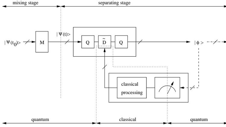
FIG. 6. Global (i.e. mixing + separating) configuration, which a feedback separating system that includes a quantum-processing inverting block and a classical-processing adapting block. Each quantum state  $|\Phi\rangle$  is used only once (no cloning): see [42].
