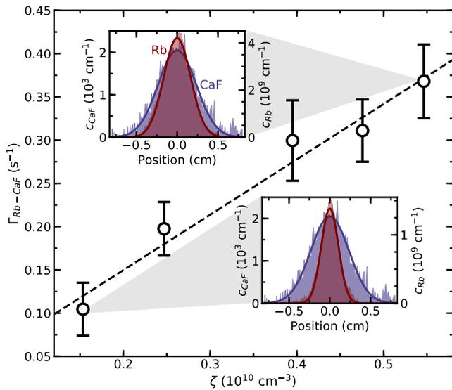
FIG. 2. Points: collisional loss rate,  $\Gamma_{\text{Rb-CaF}}$ , as a function of effective density,  $\zeta$ , for molecules in the  $|1, 2, 2\rangle$  state. Line: straight line fit to the data. Insets: radial density distributions,  $c_s(x) = \int N_s f_s(x, y, z) dy dz$ , of the atoms and molecules for small and large  $\zeta$ , with Gaussian fits.
