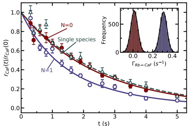
FIG. 3. Loss of molecules from the magnetic trap in the presence of  $1.2 \times 10^9$  atoms, for molecules in the  $|1, 2, 2\rangle$  state (open points) and the  $|0, 1, 1\rangle$  state (filled points). Solid lines: fits to Eq. (2). Also shown is the loss of molecules in  $|0, 1, 1\rangle$  in the absence of Rb (open triangles) together with a single exponential fit (dashed line). Inset: histogram of  $\Gamma_{\text{Rb-CaF}}$  estimates, together with fits to normal distributions.
