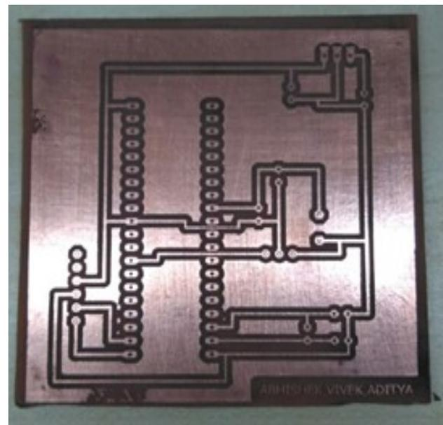
Figure 9. Printed Circuit Board after Etching process
