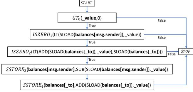
Fig. 4: An example of control and data dependency
