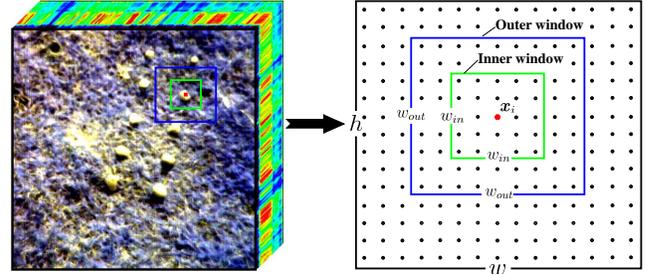
Fig. 1: The sliding dual window of the CRD.
