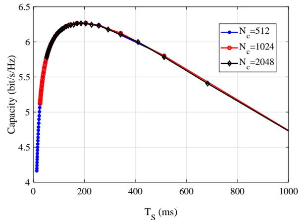
Figure 5. Spectral efficiency  $C/B$  (b/s/Hz) versus symbol length  $T_S$  for different numbers of subcarriers.
