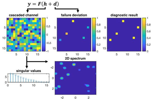
(c) Diagnosis without CSI. The cascaded channel  $\mathbf{h}$  is not low-rank anymore, but it can be sparsely represented in the 2D Fourier dictionary. Using the atomic norm as the sparsity promoter, both cascaded channel and failure mask can be recovered.
