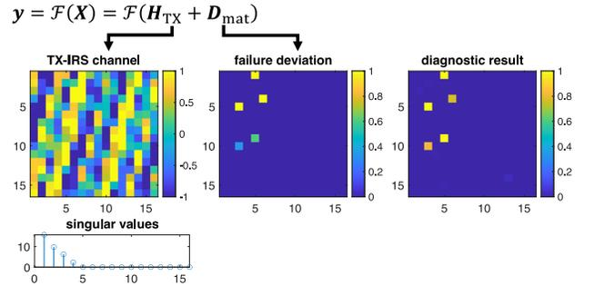
(b) Diagnosis with partial CSI. Although no reference signal is available, we can jointly exploit the low-rank property of the channel  $\mathbf{H}_{\text{TX}}$  and the sparsity of the failure deviation  $\mathbf{D}$  to recover them simultaneously.
