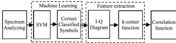
Fig. 1 : The proposed feature-based automatic modulation classification algorithm
