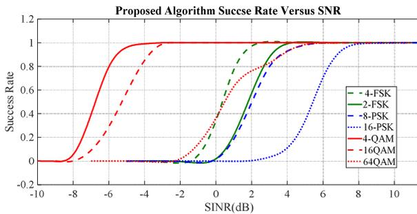
Fig. 5: Success rate of proposed algorithm in terms of SNR for different modulations.
