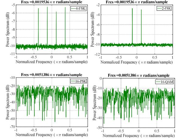
Fig. 2 : The baseband frequency spectrum of 16PSK, 16QAM, and 4FSK in the spectrum analyzer, 16QAM and 16PSK modulated signals have irregular-shape spectrum, and 4FSK modulated signal has regular-shape spectrum.
