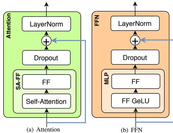
Fig. 2. Architecture of Attention and FFN blocks.
