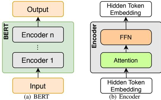
Fig. 1. Architecture of BERT and the Encoder block.
