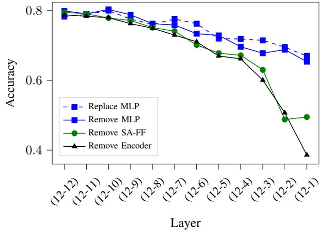
Fig. 6. Multi-layer backwards replacement/removal of different components in BERT-base, evaluated on MNLI<sub>m</sub>-sub.
