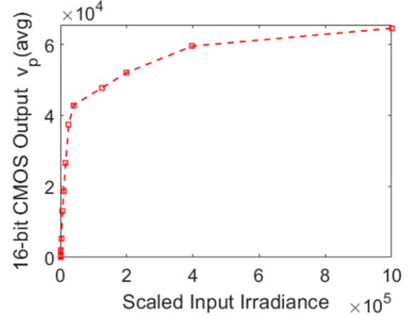
Fig. 6. Experimental CRF plot for the tested CMOS sensor-based camera.
