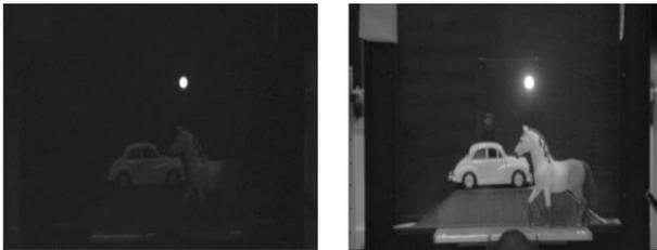
Fig. 9. Hybrid calibrated-natural 78 dB test scene images captured for the proposed minimal images multi-exposure method for HDR image recovery. Exposure times: Left image: 59  $\mu s$  and Right Image: 5.9 ms.
