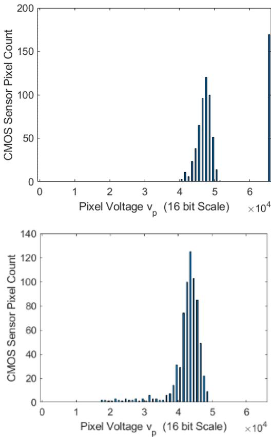
Fig. 5. Histogram plots showing the number of CMOS sensor pixels having specific 16-bit scale individual pixel range  $v_p$  signal outputs. Top plot: 14 dB DR target patch with 169 saturated pixels. Bottom plot: 28 dB target patch with no saturated pixels.
