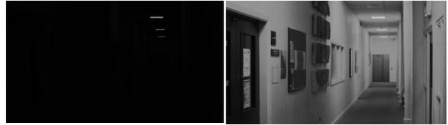
Fig. 11. Indoor natural test scene images captured for the proposed minimal images multi-exposure method for HDR image recovery. Exposure times: Left image: 888  $\mu s$  and Right Image: 88.8 ms.
