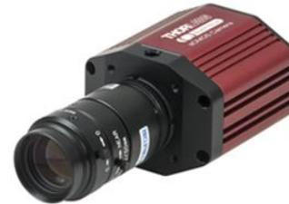
Fig. 1. Deployed 87 dB HDR CMOS-sensor based camera.
