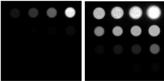
Fig. 8. 78 dB test target images captured for the proposed minimal images multi-exposure method for HDR image recovery. Exposure times are: Left image: 59  $\mu$ s and Right Image: 5.9 ms.
