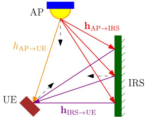
Fig. 5: Wireless links of an IRS-aided VLC system.
