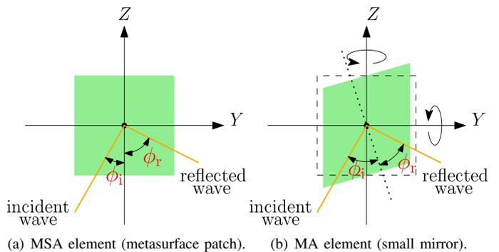
Fig. 1: Waves reflection: metasurface patch versus small mirror.
