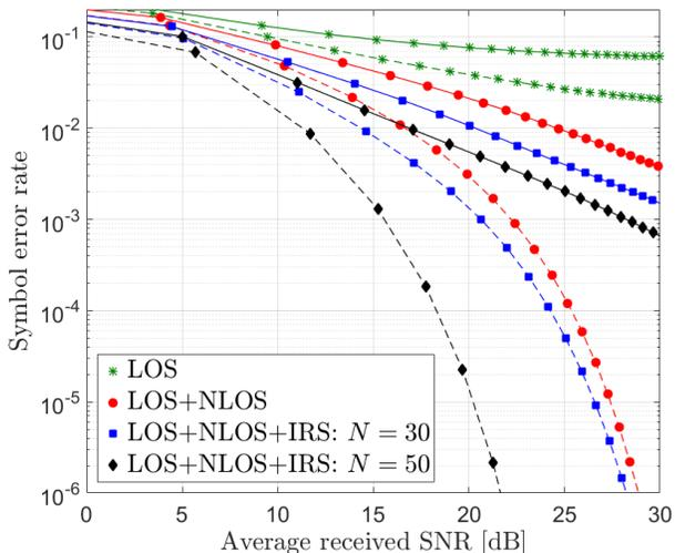
Fig. 4: SER of the OOK modulation versus the average received SNR. Solid lines represent the case when the density of blockers is  $1 \text{ m}^{-2}$  and dashed lines represent the case of a blockage-free environment.
