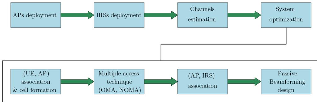
Fig. 3: Block diagram of an IRS-aided VLC System.
