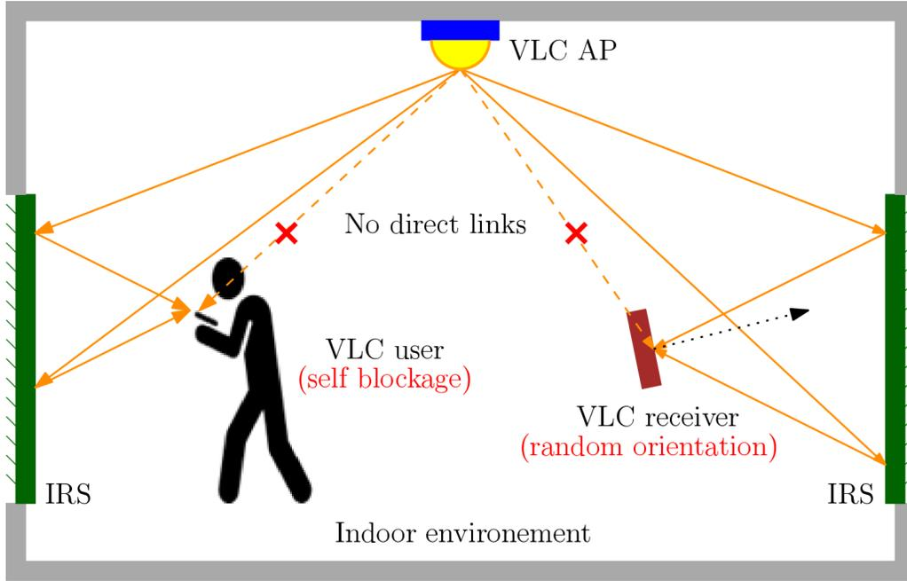
Fig. 2: IRS versus random orientation and link blockage.
