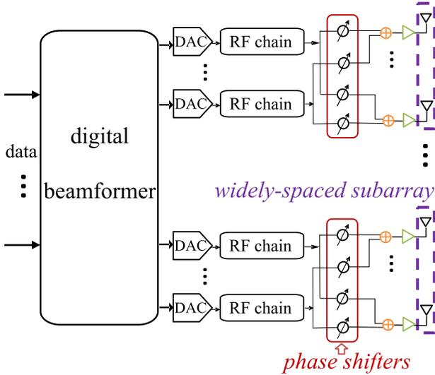
Fig. 1: The THz WSMS hybrid beamforming architecture.
