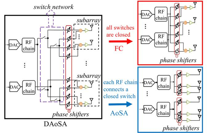
Fig. 2: The analog part of the THz DAoSA hybrid beamforming architecture.
