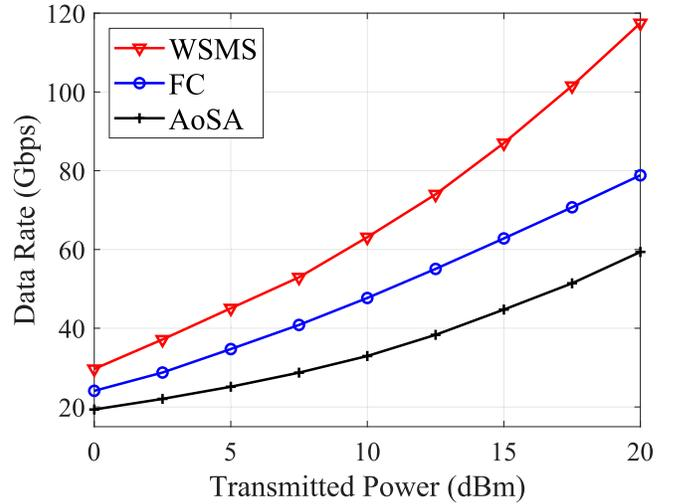
Fig. 3: The data rate of the THz WSMS, FC and AoSA architectures. The bandwidth is 5 GHz and the number of RF chains equals to 8. Two widely-spaced subarrays are arranged in the WSMS architecture.
