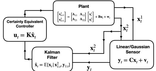
Fig. 2. The three-stage separation architecture.
