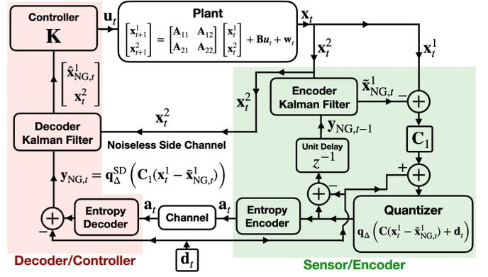
Fig. 4. The dither signal  $[\mathbf{d}_t]_i \sim \text{Uniform}[-\frac{\Delta}{2}, \frac{\Delta}{2})$  IID over  $i, t$  is independent of  $\mathbf{x}_{1:t}, \mathbf{y}_{1:t-1}, \mathbf{u}_{1:t-1}, \mathbf{a}_{1:t-1}$  but is assumed to be known at both the encoder and decoder. In practice, this “shared randomness” could be accomplished by using synchronized pseudorandom number generators at both the encoder and decoder.
