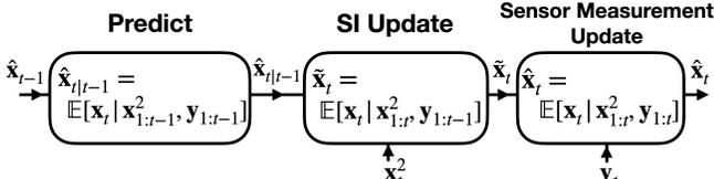
Fig. 3. A depiction of the Kalman filtering process with two measurement updates. The first update is after acquiring the SI ( $\mathbf{x}^2$ )<sub>t</sub>, meanwhile the second is after acquiring the sensor measurement  $\mathbf{y}_t$ . In the present setting, joint Gaussianity ensures the filter computes MMSE estimators. The residuals are uncorrelated, and thus independent, of the respective observations (cf. V-A).
