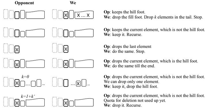
Figure 1: The function `alter`, where `deleteAny ds` generates a `Dels k xs`, and a graphical summary. Element with dotted outline are those that are considered already; the one with thick outline is the current element. It is the hill foot if it is smaller than the element to the right, or it is the last. Deleted elements are marked with a cross.
