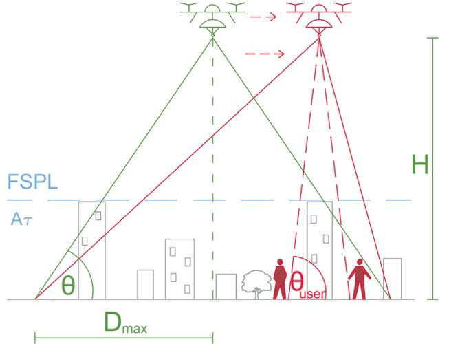
Fig. 2: Vertical mapping of the propagation environment for reference drone position (green), and a snippet of DSDSC implementation with antenna tilting (red) [3].
