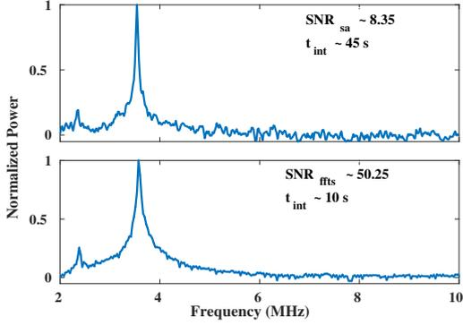
Fig. 6: Spin noise (SN) spectrum acquired from SFSA (top panel) and FFTS (bottom panel). Note that the SNR is  $\approx 50$  for the FFTS for an integration time 5x lower than SFSA. These two spectra were recorded under the same experimental conditions, at  $B_{\perp} \approx 5.1$  G.
