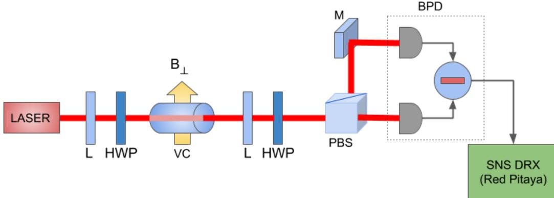
Fig. 1: A typical spin noise spectroscopy (SNS) set-up of rubidium (Rb) atomic vapor. L- plano-convex lens, VC- vapor cell (contains Rb atomic vapor), M- dielectric mirror, HWP- half wave plate, PBS- polarizing beam-splitter, BPD- balanced photodetector,  $B_{\perp}$ - orthogonal magnetic field.
