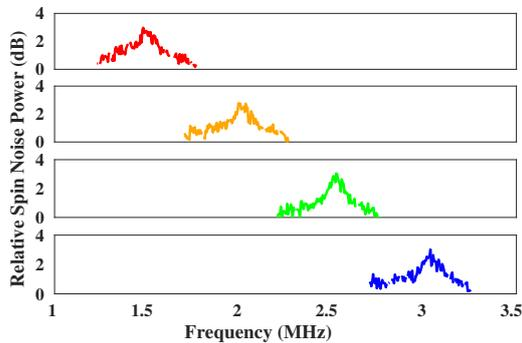
Fig. 8: Spin noise (SN) spectrum at various magnetic field strengths from the RTDR. These series of spectra has an SNR  $\approx 5$ , and the peak positions can be determined within an accuracy of  $\approx 5\%$ .
