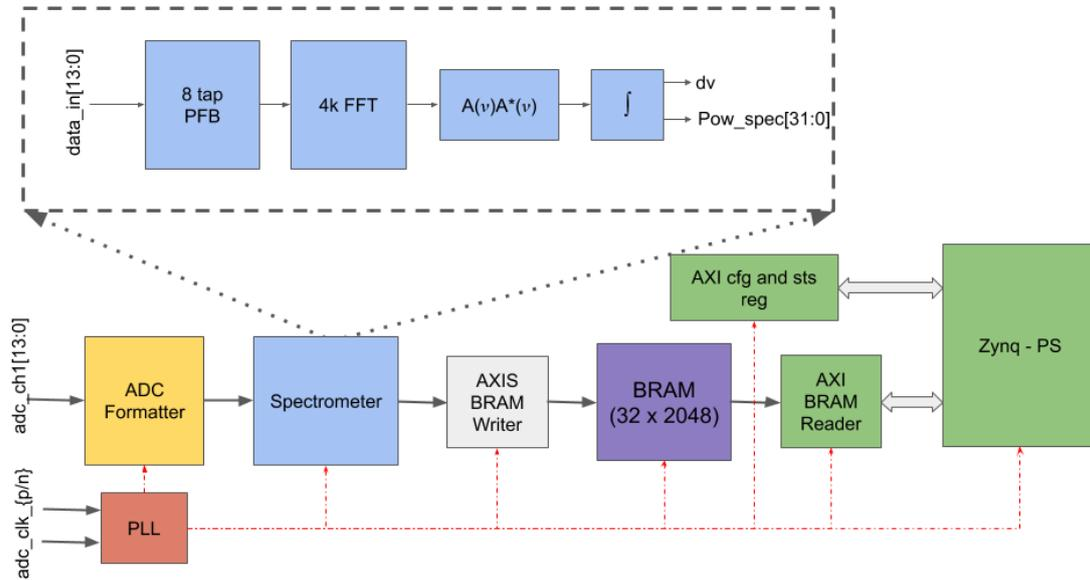
Fig. 2: Top level block diagram of the FFTS. PS and related interfaces are shown as green blocks. The red dashed lines indicate the flow of the master clock at 125 MHz, which is derived from the ADC data clock. The data and clock inputs from the ADC to the FPGA are Low Voltage Complementary Metal Oxide Semiconductor (LVC MOS) signals.
