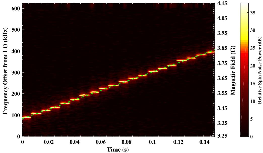
Fig. 9: Waterfall plot of the DRS output when the magnetic field was swept from  $\sim 3.35$  G to 3.85 G. We have synchronously varied the coherent drive frequency (see text). The yellow patches represent the spin noise signal in the time-frequency plane, the green dashed line is a fit to the centroids of the yellow patches and its slope indicates the rate of variation of the magnetic field in time.
