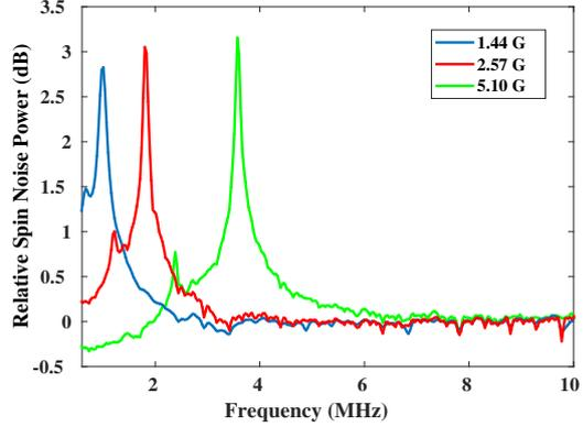
Fig. 7: Background subtracted spin noise (SN) spectra measured for different magnetic field values. The error in the measurements are  $\approx 0.02$  G, which is limited by the spectral resolution  $\approx 30$  kHz of the FFTS.
