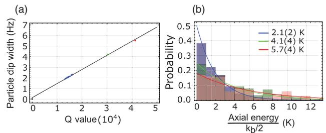
FIG. 2. (a) Explicit verification of the relationship between particle dip width and detector  $Q$  factor. (b) Axial energy distribution of a single trapped antiproton used to determine the detector temperature at three different feedback settings. The measured temperatures are shown in the figure legend.
