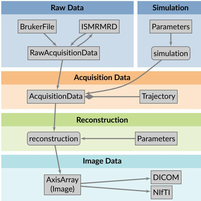
FIGURE 1 Overview of the internal architecture and the typical data flow in *MRReco.jl*. An `AcquisitionData` object can be constructed either from a file through a `RawAcquisitionData` object or using `simulation`. The `AcquisitionData` object and additional reconstruction parameters are passed to the `reconstruction` method that yields an `AxisArray` object that can be stored in DICOM or NIfTI files.
