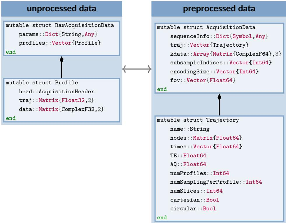
FIGURE 2 Datatypes used to represent MRI data. The left-hand side contains the julia definition of the datatype `RawAcquisitionData` used for storing unprocessed MRI data. The right-hand side contains the corresponding definition of the type `AcquisitionData` used for describing the pre-processed MRI data.
