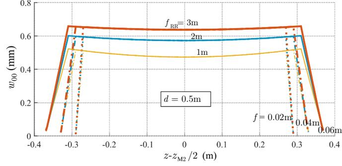
Fig. 7: Beam radius of TEM<sub>00</sub> mode along the resonator's axis for different  $f_{RR}$  and focal length  $f$  ( $z_{M2} = 2l + 2f + d$  is the resonator's length for each case)
