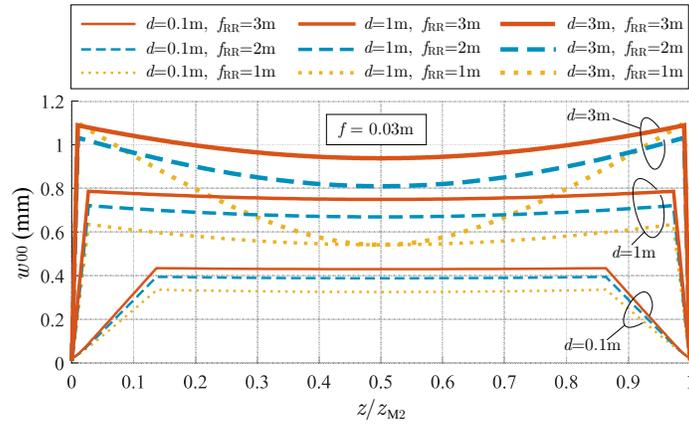
Fig. 8: Beam radius of TEM<sub>00</sub> mode along the resonator's axis for different  $f_{RR}$  and distance  $d$  ( $z/z_{M2}$  is the normalized  $z$ -coordinate, where  $z_{M2} = 2l + 2f + d$  is the resonator's length for each case)
