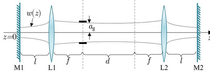
Fig. 5: Schematic of intra-cavity beam radius distribution
