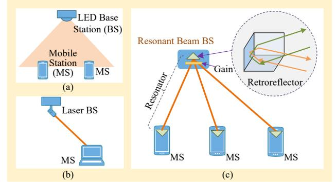
Fig. 1. Comparison of communication technologies with: (a) non-directional radiation; (b) directional radiation; (c) retro-reflective resonant beam
