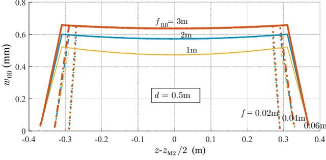
Fig. 7. Beam radius of TEM<sub>00</sub> mode along the resonator's  $z$  axis for different  $f_{RR}$  and focal length  $f$  ( $z_{M2} = 2l + 2f + d$  is the resonator's length for each case)
