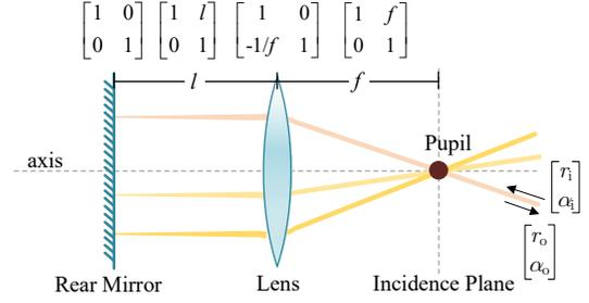
Fig. 4. Telecentric cat's eye retroreflector
