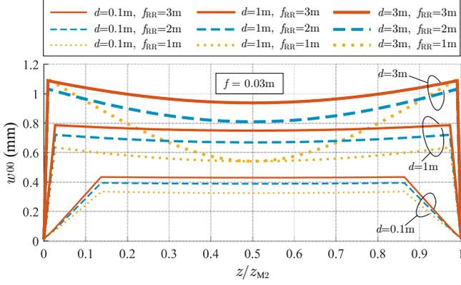
Fig. 8. Beam radius of TEM<sub>00</sub> mode along the resonator's  $z$  axis for different  $f_{RR}$  and distance  $d$  ( $z/z_{M2}$  is the normalized  $z$ -coordinate, where  $z_{M2} = 2l + 2f + d$  is the resonator's length for each case)
