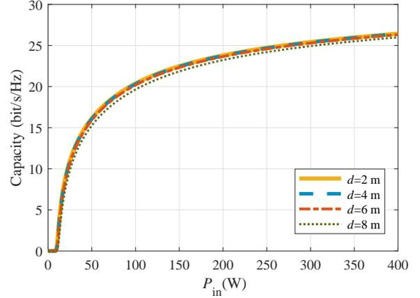
Fig. 11. Channel capacity  $\tilde{C}$  vs. electrical driving power  $P_{in}$  ( $R_4 = 0.02$ , focal length of lens  $f = 0.03$  m,  $f_{RR} = 3$  m)
