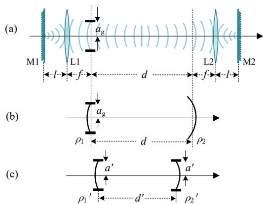
Fig. 12. Equivalent resonator for diffraction loss calculation
