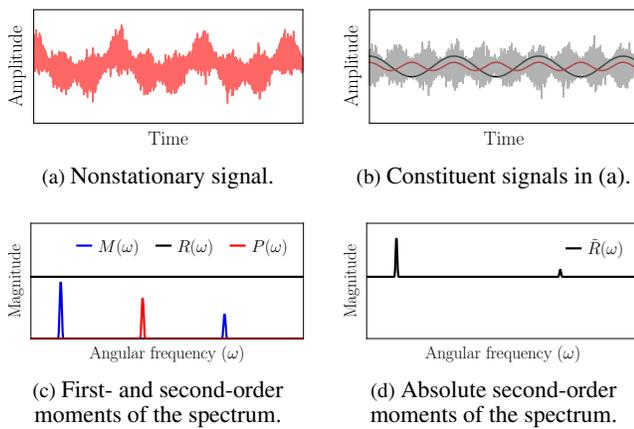
**Fig. 1:** Spectral analysis of a real-valued nonstationary signal. (a) A single realisation. (b) The constituents of the signal in (a). (c) The centred spectral moments. (d) The absolute spectral moments.
