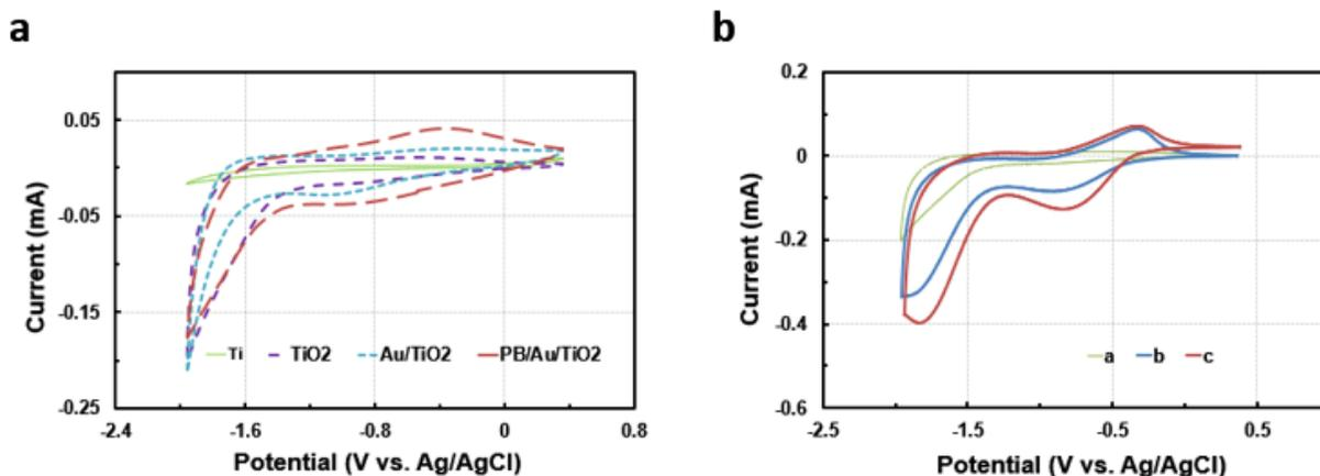
Figure 4 (a) Cyclic voltammograms of the Ti electrode (green plot) in compare with TiO<sub>2</sub> NTs electrode (purple plot), Au/TiO<sub>2</sub> NTs electrode (blue plot) and PB/Au/TiO<sub>2</sub> NTs electrode (red plot) in PBS (pH 6.0). (b) Cyclic voltammograms of the TiO<sub>2</sub> electrode (curve a) in compare with PB/Au NPs/TiO<sub>2</sub>NTs electrode in absence (curve b) and presence (curve c) of 10 mM glucose in PBS (pH 6.0).
