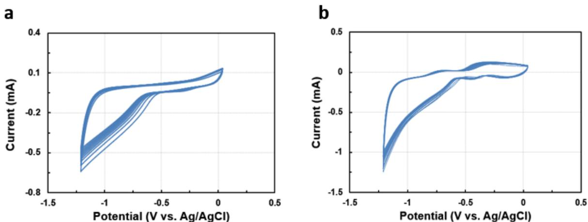
Figure 3 (a) Cyclic voltammograms of Phenylendiamine electrodeposition on PB/Au NPs/TiO<sub>2</sub> NTs electrode (b) Cyclic voltammograms of electrodeposition of GOx onto the PB/AuNP/TiO<sub>2</sub> NTs electrode via the electropolymerization of Phenylendiamine. Numerals indicated the numbers of electro polymerization cycles. Scan rate: 50 mV s<sup>-1</sup>.
