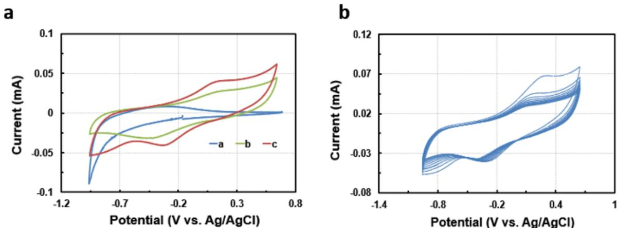
Figure 5 (a) GOx-TiO<sub>2</sub> NTs based electrode (curve a), GOx/PB/AgO NP/TiO<sub>2</sub> NTs based electrode in absence (curve b) of 10 mM glucose in PBS (pH6.0), GOx/PB/AgO NP/TiO<sub>2</sub> NTs based electrode in presence (curve c) of 10 mM glucose in PBS (pH 6.0). (b) Cyclic voltammetric behavior of the GOx/PB/AgO NPs/TiO<sub>2</sub> NTs modified electrode in presence of 10 mM glucose in PBS
