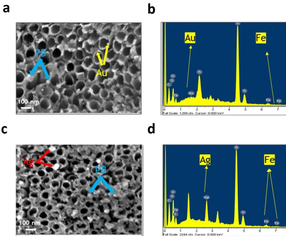
Figure 2 (a) SEM images of Au and PB nanoparticles deposited on to the TiO<sub>2</sub> NTs. (b) EDS elemental analysis. (c) SEM Images of Ag and PB nanoparticles deposited on to the TiO<sub>2</sub> NTs. (d) EDS elemental analysis
