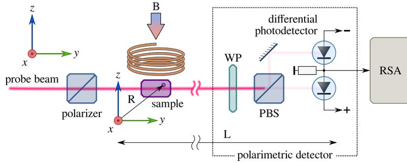
Figure 1. Schematic of the experimental setup. When observing fluctuations of the Faraday rotation, a  $\lambda/2$  waveplate (WP) was placed and used to balance photocurrents of the detector. When observing fluctuations of ellipticity, a  $\lambda/4$  WP was placed with its axes aligned at  $45^\circ$  with respect to the PBS eigen directions.
