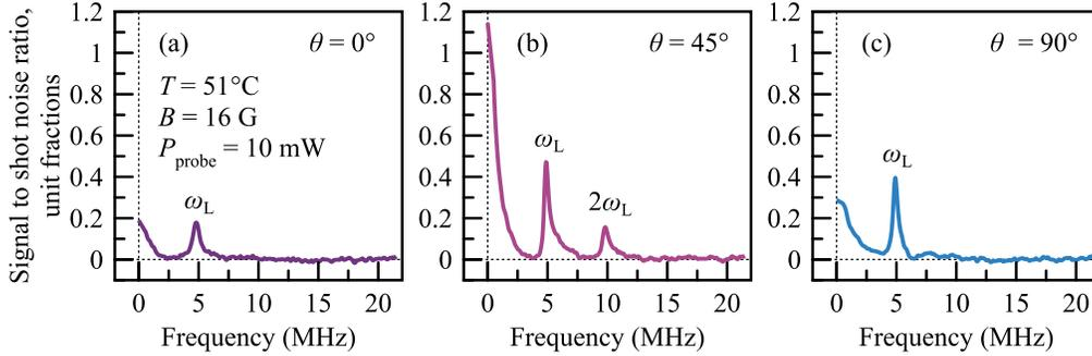
Figure 2. Ellipticity noise spectra detected at angles  $\theta = 0^\circ$  (a),  $45^\circ$  (b) and  $90^\circ$  (c) between the probe beam polarization plane and magnetic field direction. The second harmonic of the Larmor frequency is well pronounced at  $\theta = 45^\circ$  and vanishes at  $\theta = 0$  and  $90^\circ$ .
