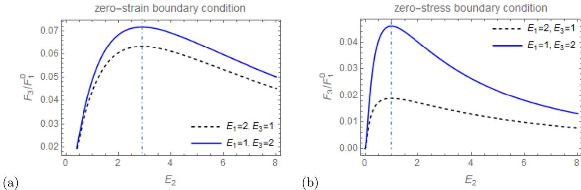
Figure 2: Transferred energy to the load  $F_3$  normalized by initial energy of active component  $F_1^0$  as a function of  $E_2$  with  $M = 2, r_2 = 2, r_3 = 3$ . The vertical dot-dashed lines are located at the optimal value of  $E_2$  (a.u.), given by Eq. (17) and Eq. (19), respectively. (a) zero-strain boundary condition, (b) zero-stress boundary condition.
