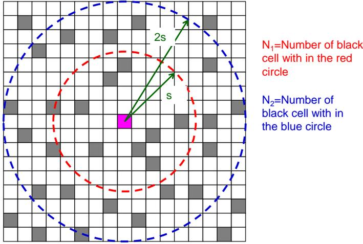
**Figure 3.** Schematic diagram of the summing of states  $N_1$  and  $N_2$ . Each grid cell has state 0 (white) or 1 (black). The inner area has a domain within  $s$  grids of the focal cell and the outer area has a domain within  $2s$  grids.
