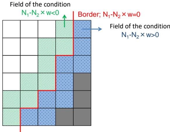
Figure 5. Example of the situation of the boundary between black cell (state 1) and white cell (state 0); Black cell (1) in contact with white cell (0) has  $N_1 - N_2 w > 0$ , and white cell (0) in contact with black cell (1) has  $N_1 - N_2 w < 0$ .
