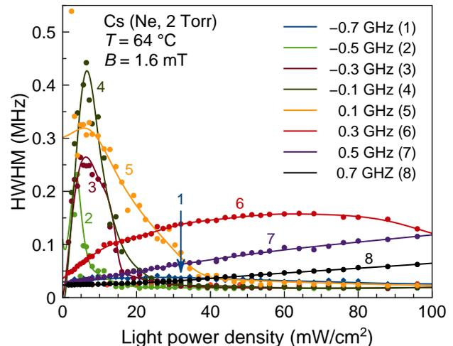
Figure 4. Dependence of the SN resonance width on the probe beam intensity at different detunings of the probe light frequency from the center of the Doppler-broadened transition  $F = 4 \leftrightarrow F' = 3, 4, 5$  of cesium.
