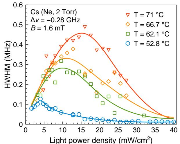
Figure 8. The width of the “wide” component of the SN resonance as a function of the probe light intensity at different temperatures:  $T = 71$  °C (triangles),  $T = 66.7$  °C (diamonds),  $T = 62.1$  °C (squares), and  $T = 52.8$  °C (circles). The solid lines are a guide to the eye.
