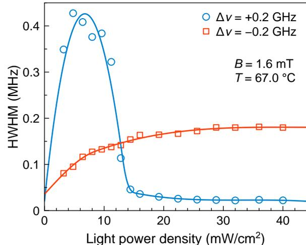
Figure 6. Example of the same dependence as in Fig. 4, but obtained on the transition from the lower HF component of the ground state ( $F = 3$ ). The symbols represent the data measured at  $+0.2$  GHz (circles)  $-0.2$  GHz (squares) detunings. The solid lines are a guide to the eye. The sides of the transition with higher and lower sensitivity to optical perturbation of the ground-state spin-system are interchanged.
