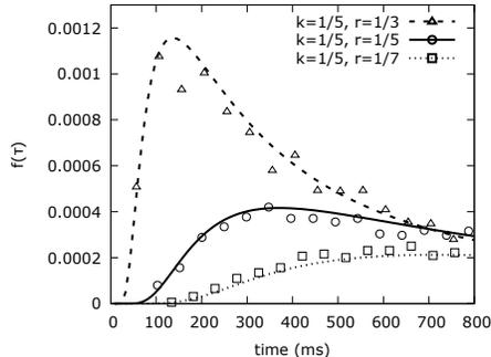
Figure 3: **First-passage-time distributions** for different noise colouring obtained by numerical simulation of (13) (scatter plots) together with the theoretical approximation  $f_{r \neq k}(t)$  (lines) for some different parameters (indicated by different line types). Parameter values not mentioned in the legend are  $x_c = 1$ ,  $x_r = -3$  and  $\sigma = 0.05$ . The numerical results are from 20000 neurons per line simulated for 25000 time-steps of size  $\Delta t = 0.1$
