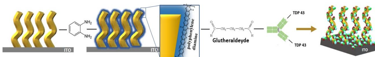
**Figure 1.** Scheme of the sensing device and functionalization protocol. The core-shell architecture arises from covering the fabricated helix array with the P-oPD insulating polymer. Then, the antibody is immobilized onto the shell after crosslinking by glutaraldehyde. Finally, the target analyte, deposited on the sample surface, is recognized by the specific antibody sites in dry environment.
