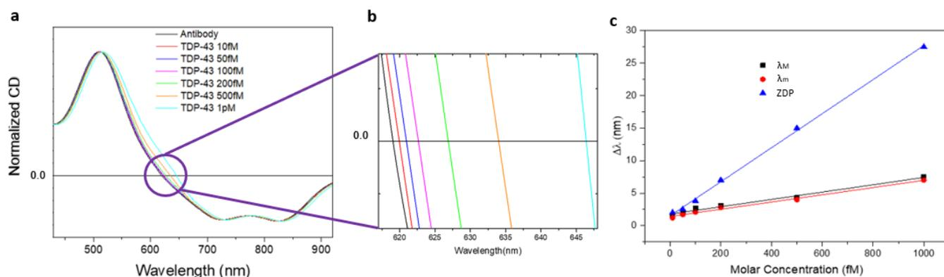
**Figure 5.** a. Normalized CD spectra acquired after the only deposition of the antibody layer (spectral reference) and after different concentrations of TDP-43; b. the high-magnification around the ZDP region allows to evaluate the spectral shift of the crossing point between antibody and the antigen at different molar concentrations; c. Linear fit of the spectral shift for  $\lambda_M$ ,  $\lambda_m$  and ZDP respectively. The size of data points represents the error bars.
