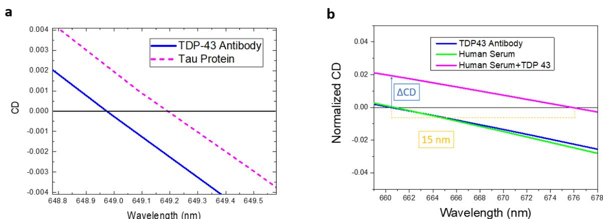
**Figure 6.** a. Detailed plots of the ZDP for CD spectra acquired after the incubation of TDP-43 antibody (blue curves) and Tau protein (pink dashed line). As depicted by ZDP position, no significant changes are recorded b. Detailed plots of the ZDP for CD spectra measured after the incubation of TDP-43 antibody (blue curves), human serum only (green line) and human serum + TDP 43 (pink lines). Large spectral shift of 15nm is observed only in presence of the target antigen.
