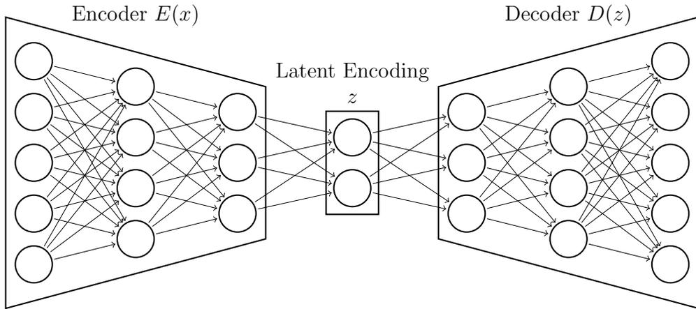
**Exhibit 2:** An autoencoder can be split into encoder and decoder networks. Note that the dimensionality of the latent encoding is typically smaller than the original input dimension.
