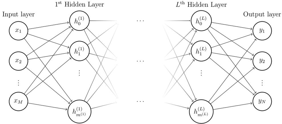
**Exhibit 1:** A neural network with  $L$  hidden layers, with  $M$  inputs and  $N$  outputs. The  $i^{\text{th}}$  hidden layer contains  $m^{(i)}$  neurons, and  $h_k^{(i)}$  is the value at the  $k$ th neuron of hidden layer  $i$ .
