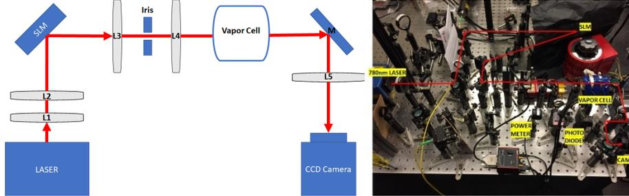
Fig. 3. Experimental setup. (a) Cartoon layout of the setup. The focal lengths of the lenses are: L1 = 50 mm; L2 = 300 mm; L3 = 150 mm; L4 = 150 mm; L5 = 100 mm. M indicates a flat mirror. (b) Photograph of the experiment.
