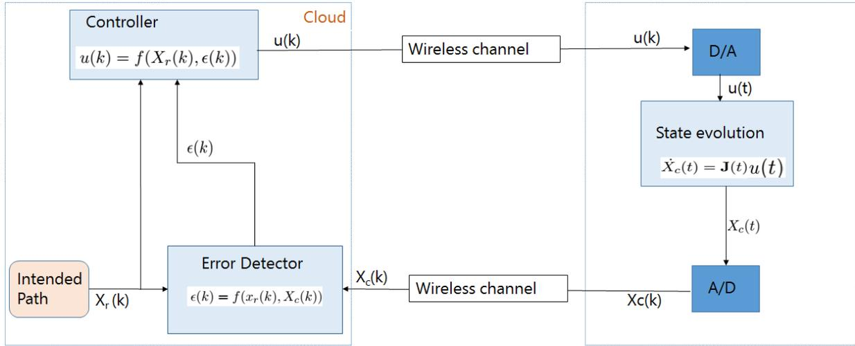
Figure 1: Discrete system of Cloud Controlled AGV
