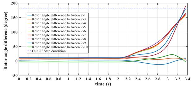
Fig. 5 Rotor angle difference of generators during 2-phase fault
