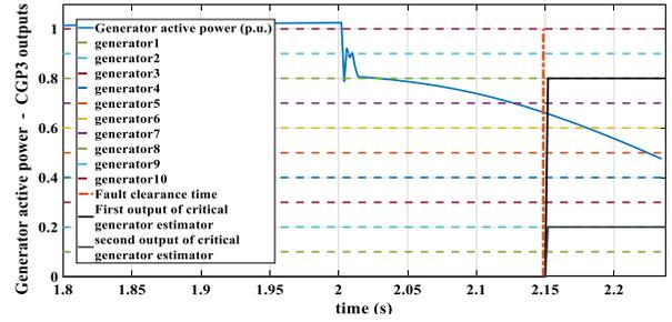
Figure 4. Output variation of critical generator predictor function for a random 2-phase fault.
