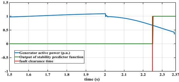
Figure 3. Output of stability predictor function for 3-phase fault
