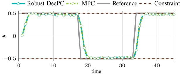
Fig. 1: Comparison of the Robust DeePC and the MPC controller. Note that the two responses are the same.
