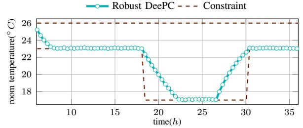
Fig. 2: Temperature control with robust DeePC
