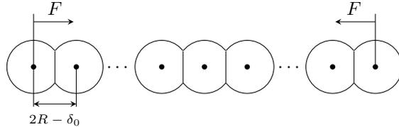
Figure 1: Schematic illustration of a particle chain with precompression. The chain consists of  $N$  identical, aligned spheres with radius  $R$ . The interaction potential between adjacent spheres is governed by (2). Applying a compressive force  $F$  at both ends of the chain compresses each sphere at the contact point by a uniform distance  $\delta_0$ .
