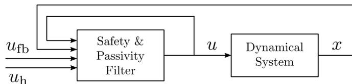
Fig. 1: Passivity and safety filter: the human input  $u_h$  the state feedback controller  $u_{fb}$  are modified by a filter before being supplied to the dynamical system (e.g. a teleoperated robotic system) in order to ensure its safety and passivity.
