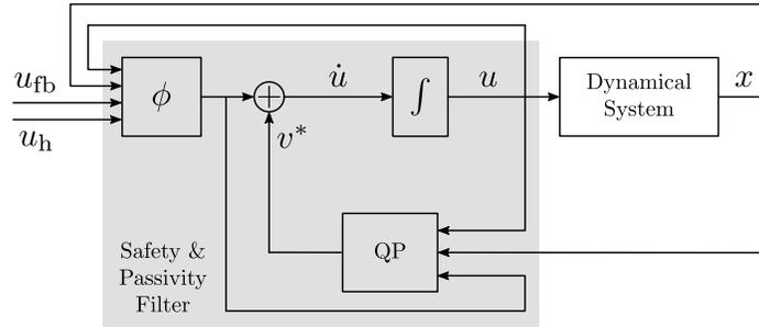
Fig. 2: Passivity and safety filter: the structure of the filter depicted in Fig. 1 is specified using the results of the paper. The filter includes the computation of the function  $\phi$ , whose expression is given in (20), the solution of the convex quadratic program (QP) (25), and an integration step, in order to compute the control input  $u$  supplied to the system.
