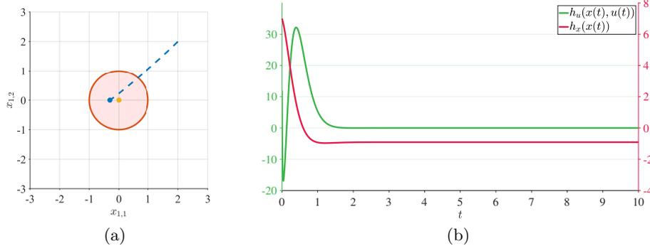
Fig. 3: Trajectory (Fig. 3a) and passivity I-CBF (Fig. 3b) for the system (27) controlled using  $v(t) = 0$  for all  $t$ . The state  $x_1$  converges to  $[x_{1,1}, x_{1,2}] = [-0.3, 0]$  as expected, however both the safety and the passivity conditions are violated. In fact, the blue point enters the unsafe region shaded in red in Fig. 3a, and both  $h_u$  and  $h_x$  take negative values in Fig. 3b.
