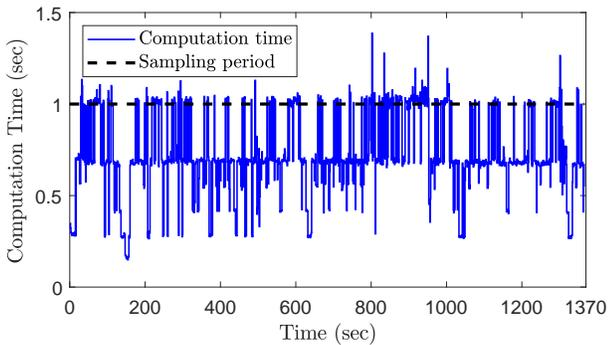
Fig. 3. The computation time for obtaining our numerical solution at each time instant over the UDDS driving cycle.
