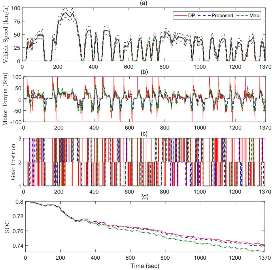
Fig. 2. Simulation results for the UDDS driving cycle with planning horizon  $N = 8$ : (a) vehicle speed trajectories, (b) motor torque trajectories, (c) gear position trajectories, and (d) battery  $SOC$  trajectories.
