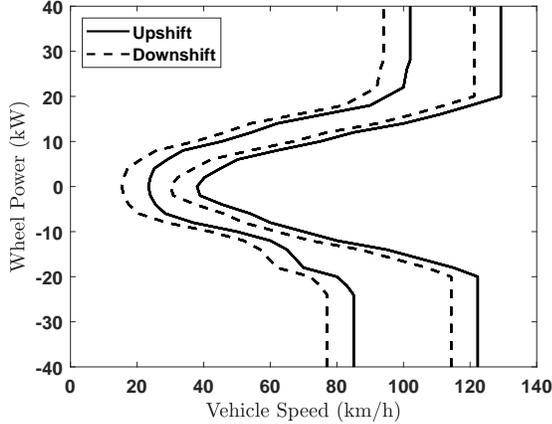
Fig. 1. Gear shift map optimized through the approach of [35].
