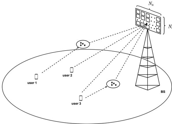
Fig. 4. Uplink transmission in the multi-user massive MIMO system.
