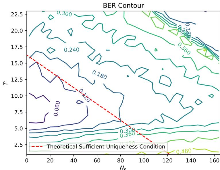
Fig. 9. BER contour in  $(N_s, T')$  plane in testing stage
