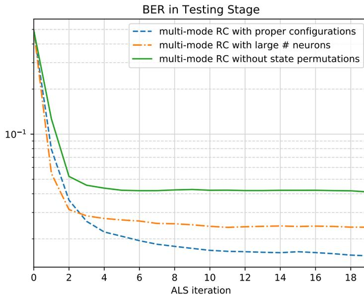
Fig. 7. Testing BER of Multi-Mode RC with respect to iterations in ALS.
