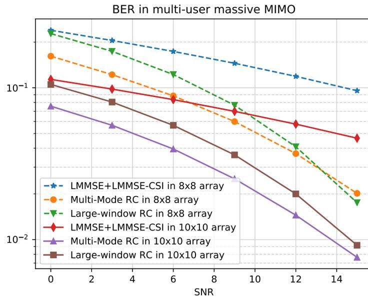
Fig. 11. BER in multi-user massive MIMO with 64 ( $8 \times 8$ ) and 100 ( $10 \times 10$ ) antennas at the BS.
