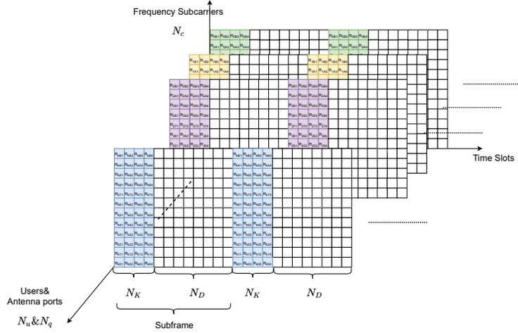
Fig. 5. Massive MIMO-OFDM resource grids (subframe-subcarrier) structure for RC training and symbol detection
