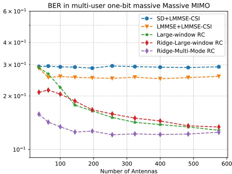
Fig. 12. BER in one-bit multi-user massive MIMO systems with different antenna numbers.
