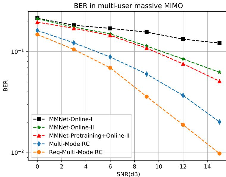
Fig. 13. BER in a multi-user massive MIMO system with 64 antennas at the BS ( $8 \times 8$  antenna array).
